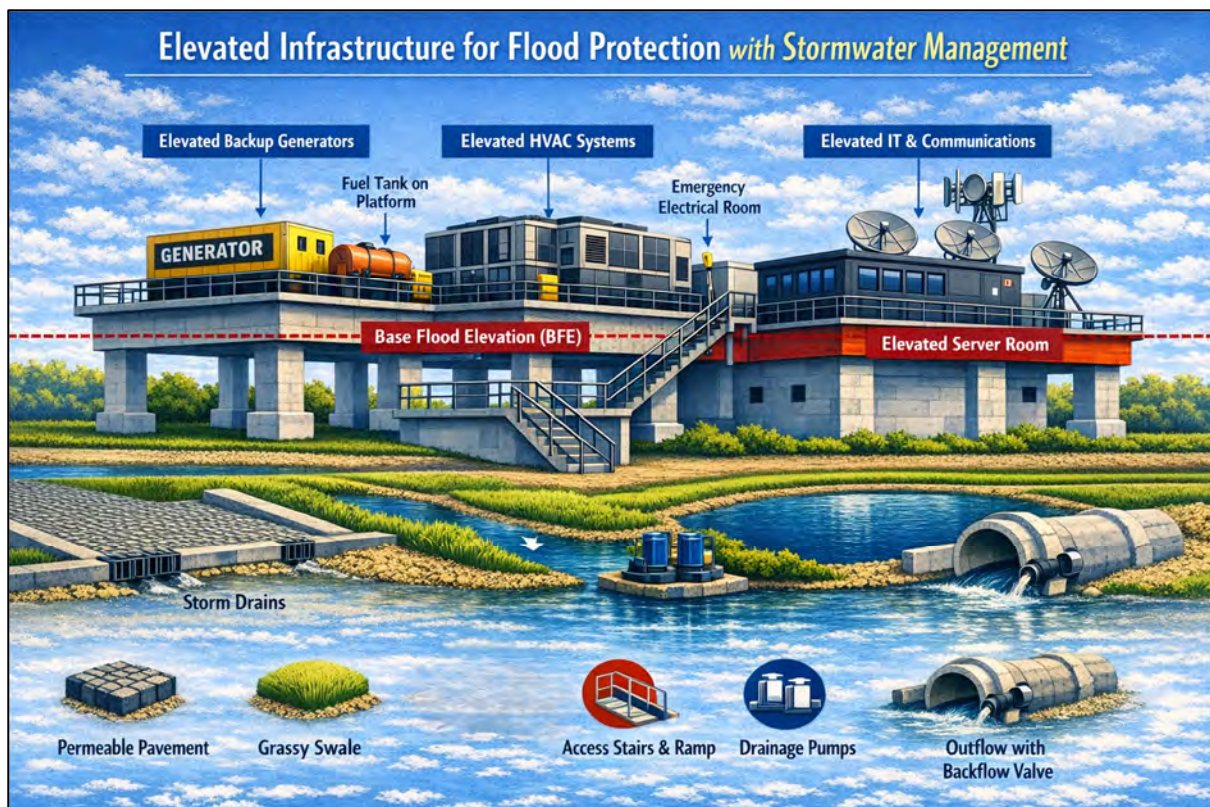
Figure 5: Examples of Site-Level Flood Protection Stormwater Retrofits
