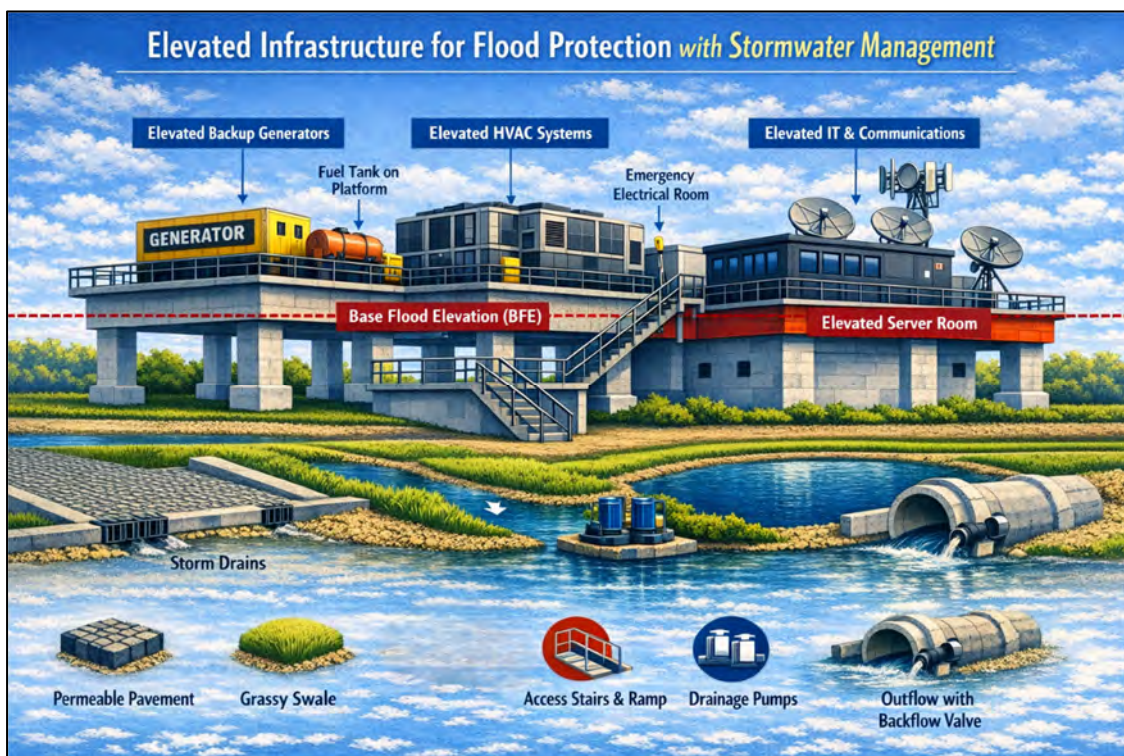
Figure 5: Examples of Site-Level Flood Protection Stormwater Retrofits
