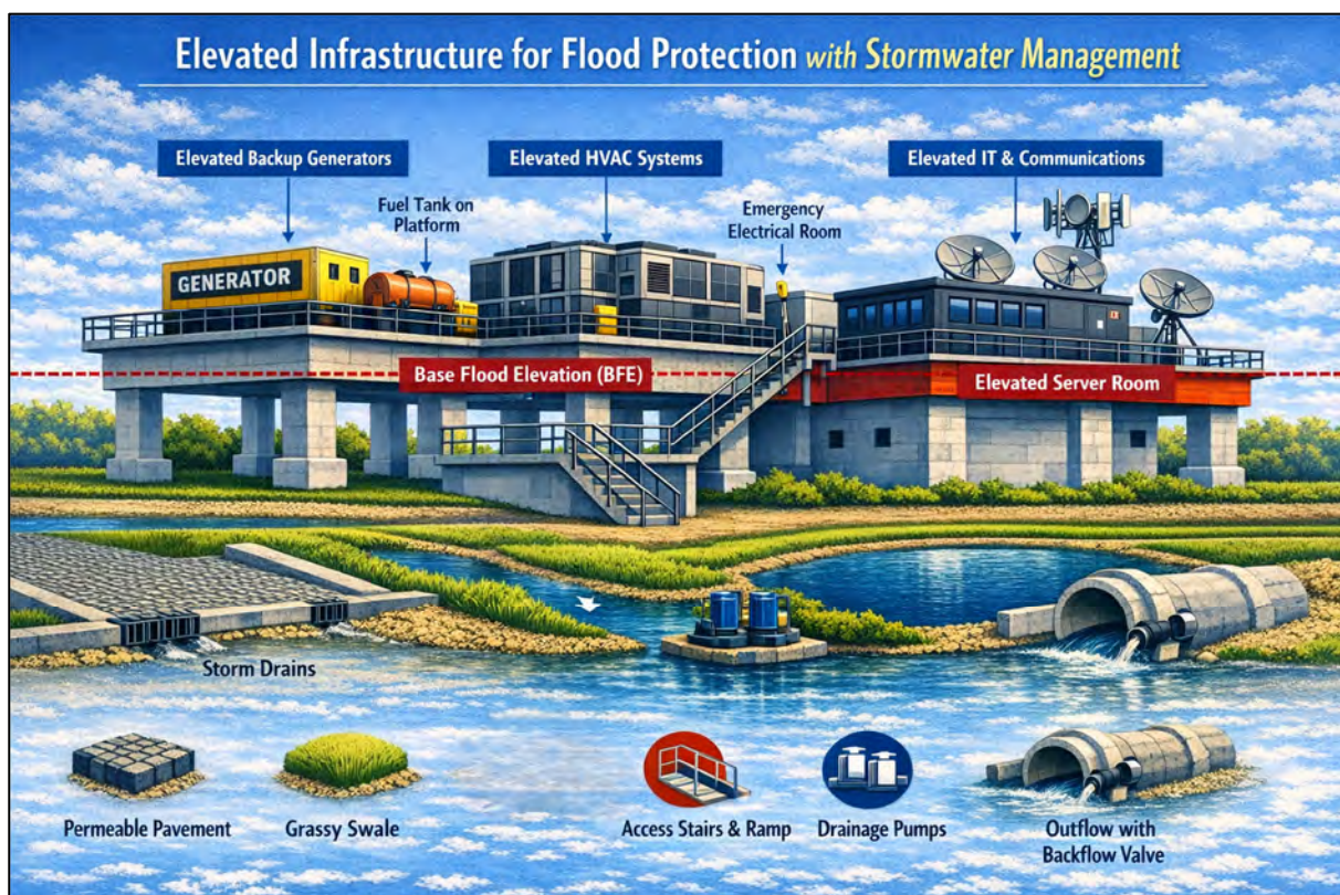
Figure 5: Examples of Site-Level Flood Protection Stormwater Retrofits
