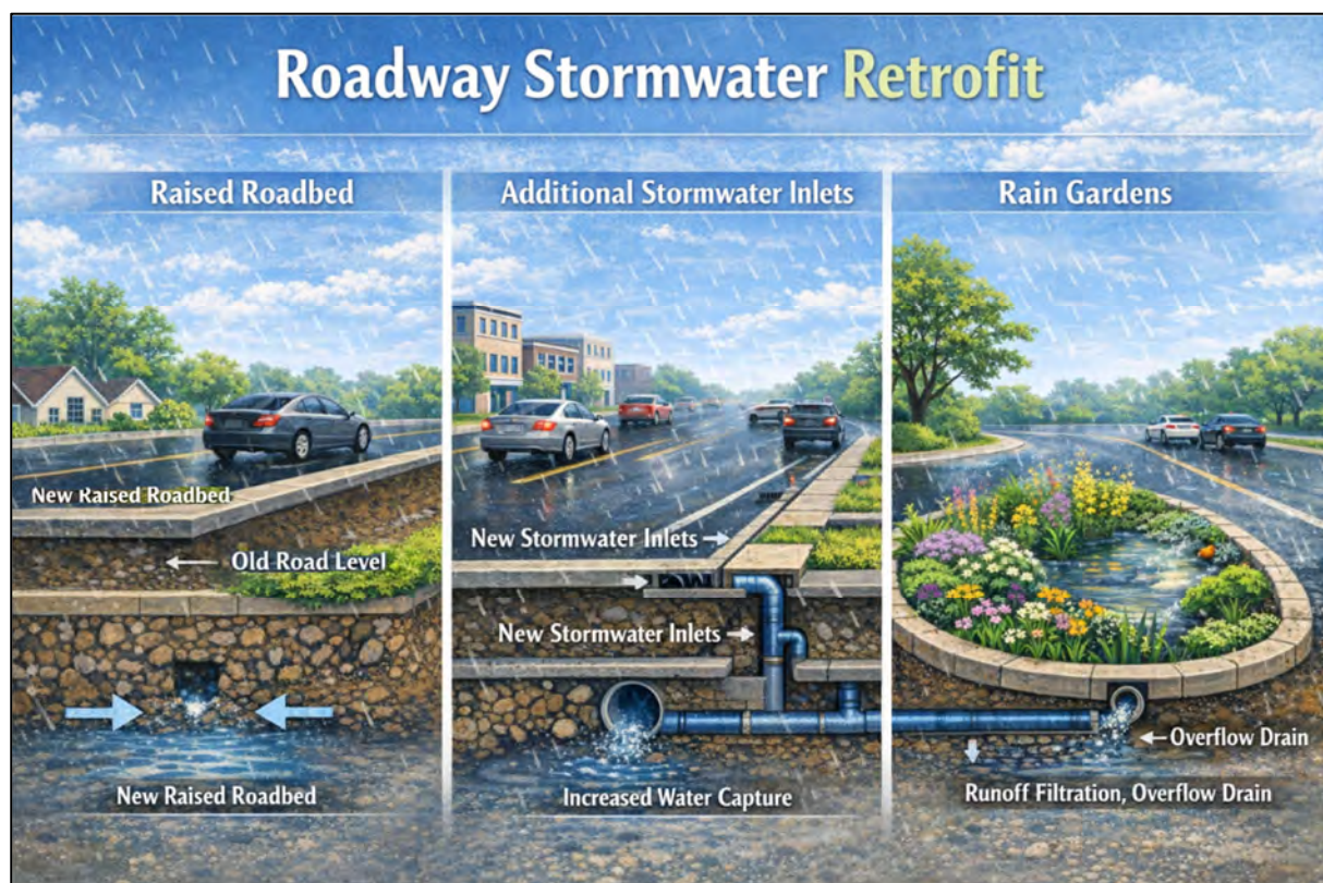
Figure 4: Examples of Roadway Stormwater Retrofits
